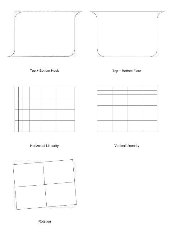
Figure A-2: Hook, Flare, Linearity, and Rotation Distortion
