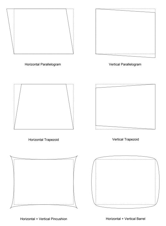
Figure A-1: Parallelogram, Trapezoid, Pincushion, and Barrel Distortion
